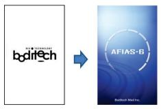
During system initialization, AFIAS-6 will display each test items and the test results will be displayed. After finishing this step, AFIAS-6 will display the mode selection window. If a user does not select a test mode within 10 seconds, the test mode is set to 'General mode' by default. Then AFIAS-6 will display the log-in window. If there is any problem, an error message is displayed. If a user taps the 'Confirm' button, AFIAS-6 will be ready for testing.
